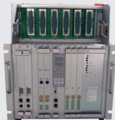
▲ TCMS Train control and monitoring system (TCMS)
