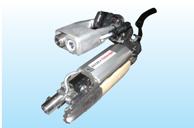
PCV内部遠隔調査ロボット Remote-controlled robot for internal primary containment vessel (PCV) investigation
