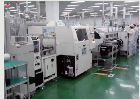
Production line for ECUs for EPS systems
