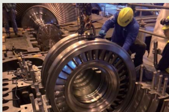
High-pressure turbine rotor for Ottumwa Generating Station, U.S.A.
