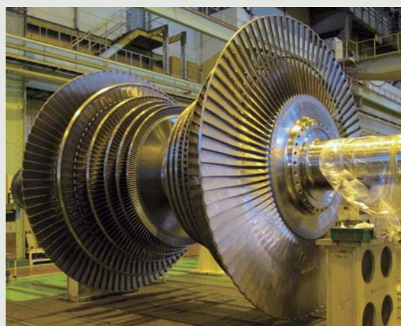
Low-pressure turbine rotor for Kudgi Super Thermal Power Plant Unit 1, India
