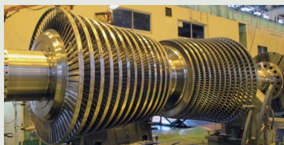
Intermediate-pressure turbine rotor for Kudgi Super Thermal Power Plant Unit 1, India
