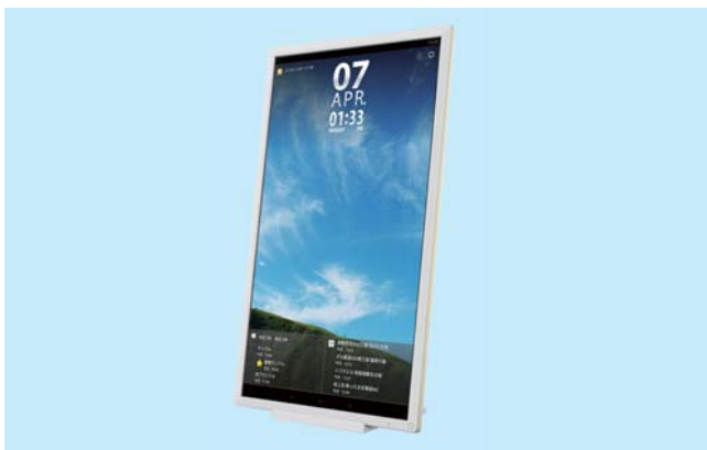
シェアードボード Shared Board 10-point touch display with 24-inch electrostatic capacitance type panel
