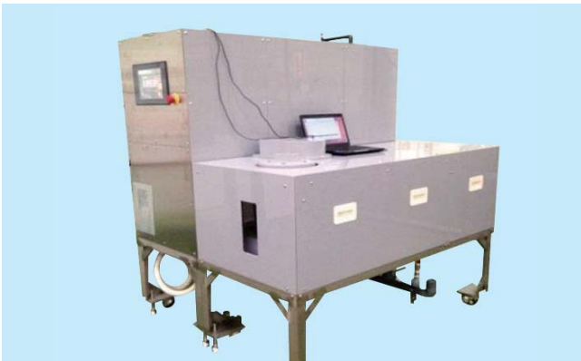
有隔壁3室型セルを採用した電解機能水生成装置 Electrolyzed functional water generating system using three-chamber type electrolyzer with two separators
