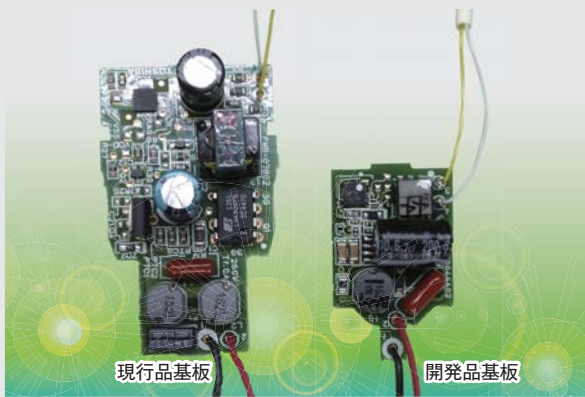
▲ 現行品と開発品の基板サイズの比較 Comparison of overall size of conventional and newly developed printed circuit boards
