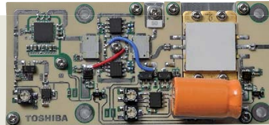
Compact high-power generator for portable microwave surgical instruments
