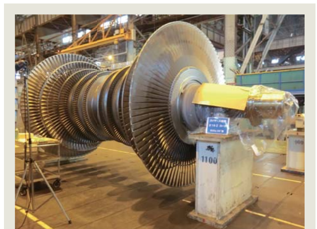
Second-generation super-rotor for Unit 19-2 of Calistoga Geothermal Power Plant, U.S.A.
