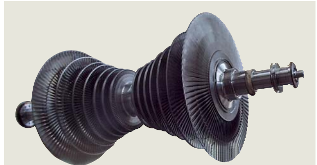
Turbine rotor for Olkaria Geothermal Power Station, Kenya
