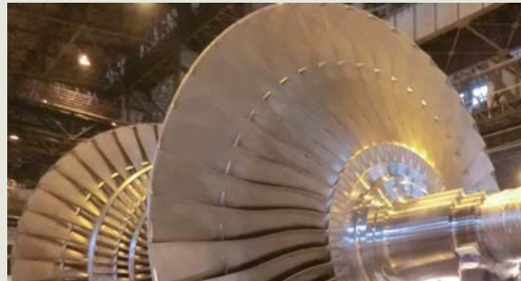
Low-pressure (LP) turbine rotor
