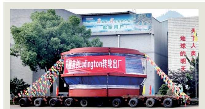
Replacement pump-turbine runner for Ludington Pumped Storage Power Plant, U.S.A.
