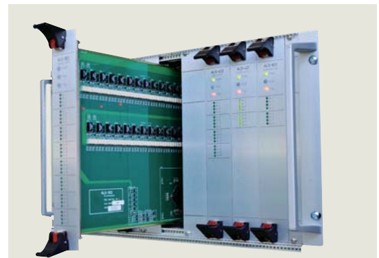
I&C platform for safety systems using FPGA technology
