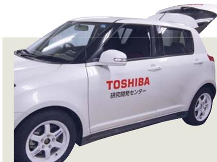
EV incorporating 7 kW wireless power transmission system
