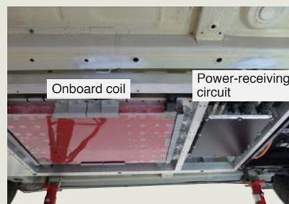
Coil and power-receiving circuit installed on underside of EV
