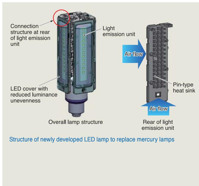
Structure of newly developed LED lamp to replace mercury lamps
