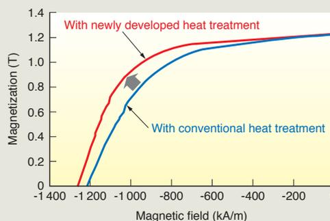
Demagnetization curves of SmFeCo magnets
