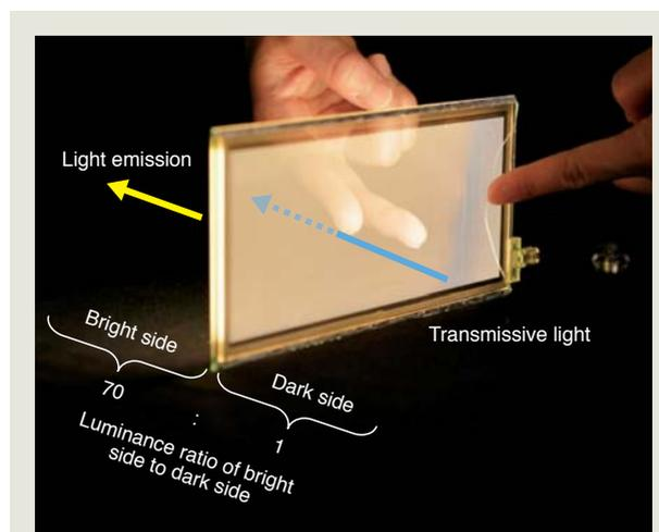
Transmissive one-side-emission OLED panel
