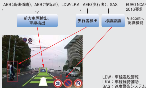
▲ Euro NCAP 2016 に対応するVisconti™の認識機能 Recognition features of Visconti series general-purpose image recognition processor compliant with Euro NCAP (European New Car Assessment Programme) 2016
