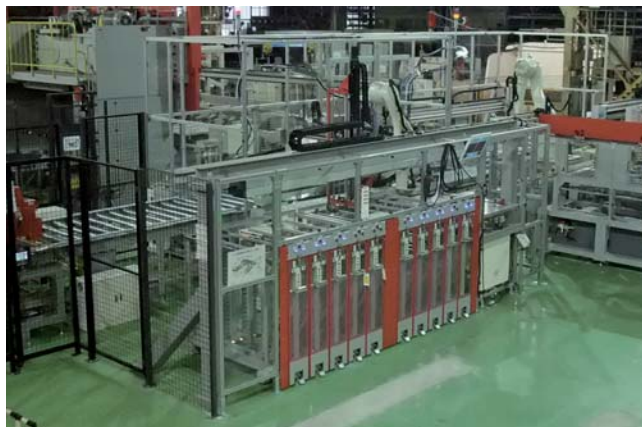
板金パネル部品の自動組立設備 Parts assembly equipment for elevator automatic production line
