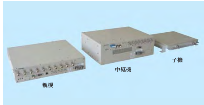
LTE 対応マルチバンド屋内用 通信エリア拡張システム Multiband distributed antenna system for indoor coverage of Long Term Evolution (LTE) mobile phone base transceiver stations
