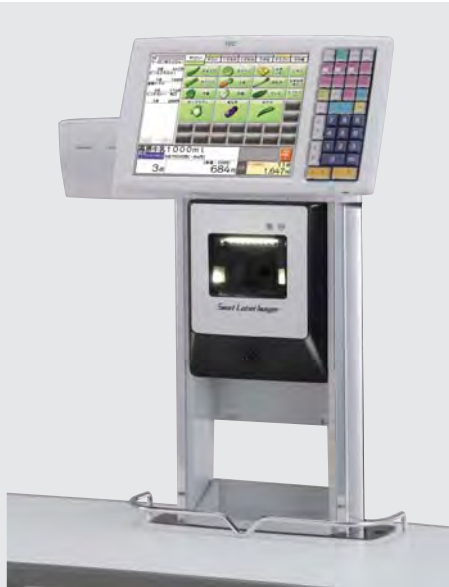
▲ IS-890T IS-890T vertical barcode scanner with image processing technology
