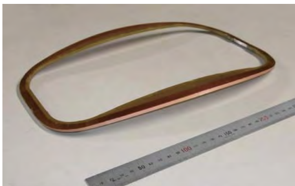
3次元形状のY系超電導コイル Three-dimensional (3D)-shaped yttrium barium copper oxide (YBCO) coil
