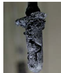
Dy metal recovered on electrode using molten-salt electrolytic deposition
