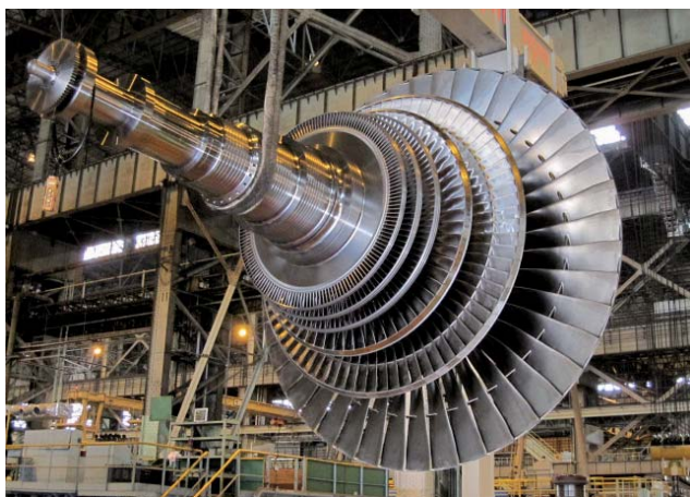
Low-pressure turbine rotor applying 48-inch titanium last-stage blade
