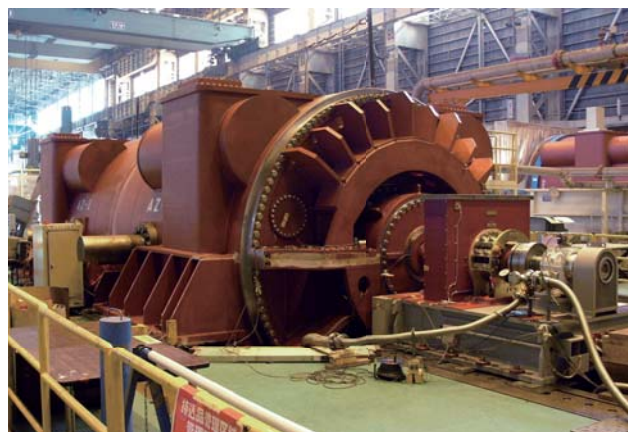
670 MVA indirectly hydrogen-cooled turbine-driven generator undergoing shop test
