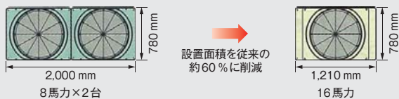
▲ 16馬力室外機の設置スペース Comparison of footprints of two 8 HP outdoor units and one 16 HP outdoor unit
