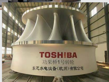
▲ 現地ランナ製造工場と現地溶接ランナ Runner manufacturing factory at site and on-site-welded runner
