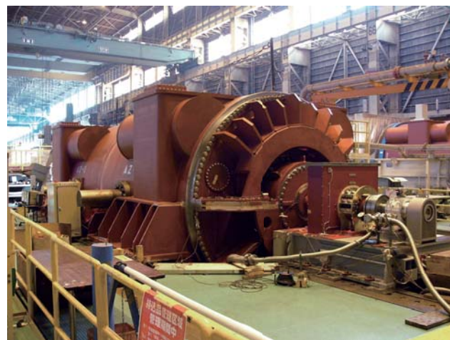
670 MVA indirectly hydrogen-cooled turbine-driven generator undergoing shop test
