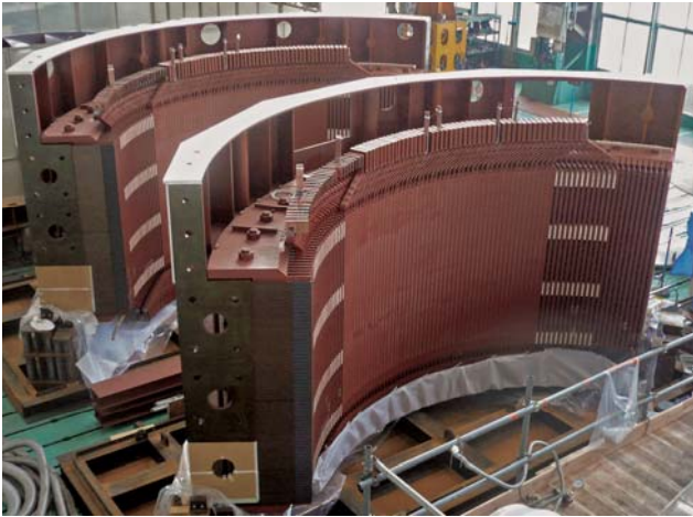
Section of generator stator for Porce III Hydroelectric Power Plant, Colombia
