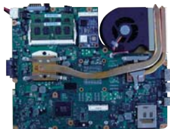
Integration of system board and SpursEngine sub-board for Qosmio V65/F60
