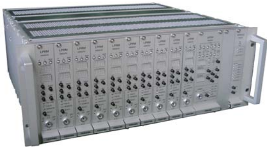
Neutron monitor using FPGAs
