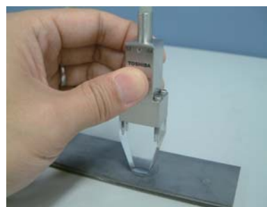
Probe for spot weld inspection
