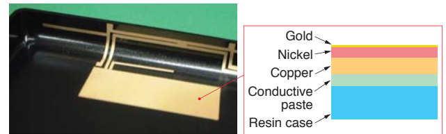
Antenna formed directly on resin case
