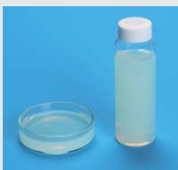
◀ 光触媒ナノ粒子の水系分散液 Aqueous dispersion slurry of photocatalyst
