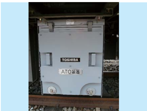
ATO制御装置 Automatic train operation (ATO) equipment
