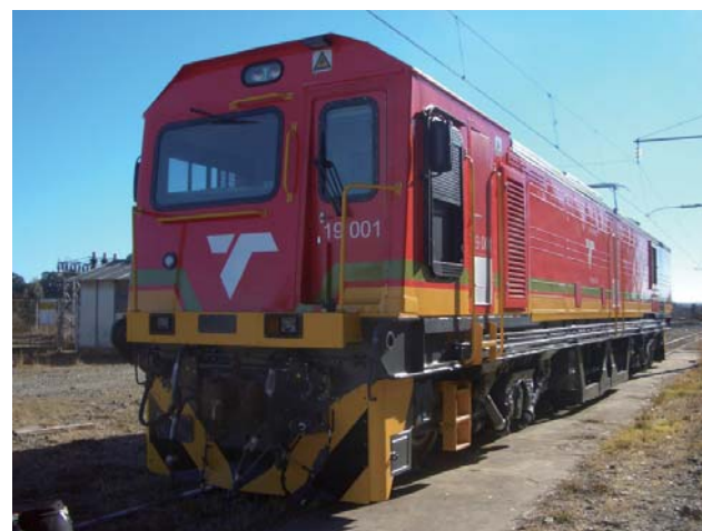
25 kVac/3 kVdc dual voltage electric locomotive in South Africa
