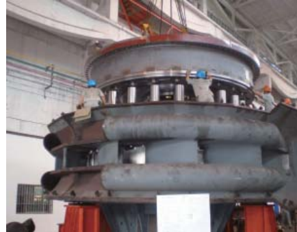
Shop assembly of turbine stationary parts for Dayingjiang Power Plant, China
