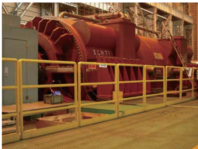
1000 MW generator at shop test
