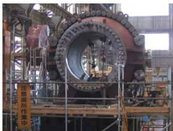
Factory assembly of inlet valve for Xilongchi Pumped Storage Power Station
