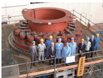
Factory assembly of pump-turbine for Xilongchi Pumped Storage Power Station
