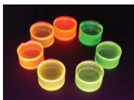
Application of novel compounds Rare-earth organic luminescent compounds dissolved in polymer
