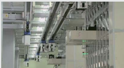
▲ 製造装置へのウェーハ自動搬送 Automated system for transporting wafers between manufacturing stages
