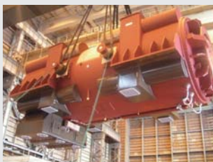
▲ 発電機出荷状況 Shipment of generator from factory
