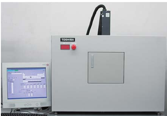
LIBS法を用いたレーザー堆肥分析装置 GeoRight™ GeoRight™ compost analyzer using laser-induced breakdown spectroscopy (LIBS)
