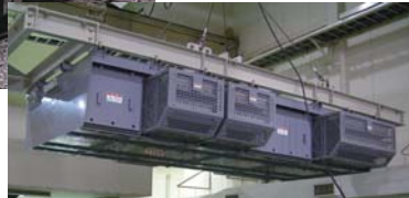
TRA700形電車と主変換装置 TRA series 700 electric train and main converter
