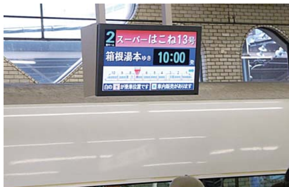
小田急電鉄(株)向け 特急乗車案内装置 Boarding information display for "Romancecar" limited express trains of Odakyu Electric Railway Co., Ltd.
