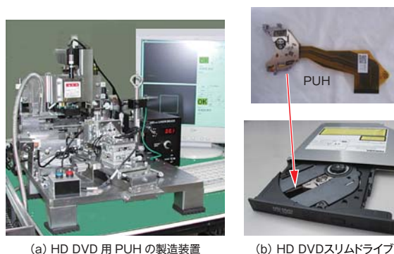
HD DVD用PUHの製造装置とノートPC搭載用薄型ドライブ Pickup head (PUH) manufacturing equipment for HD DVDs (left) and HD DVD slim drive for notebook PCs (right)
