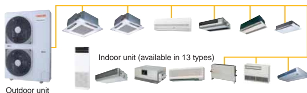
Configuration of the “Mini-SMMS™” system
