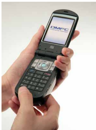
Prototype DMFC-powered cellular phone (jointly developed with KDDI)
