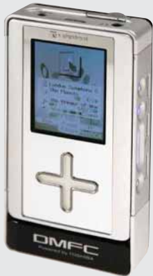
▲ 燃料電池駆動 gigabeat™ (試作機) Prototype DMFC-powered gigabeat™
