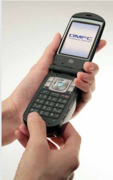
▲ 燃料電池駆動携帯電話 (試作機：KDDI (株)との共同開発品) Prototype DMFC-powered cellular phone (jointly developed with KDDI)
