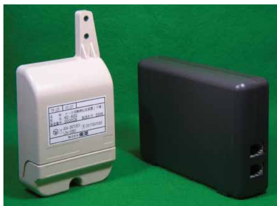
自動検針用無線ユニット (無線子機 RD-60G (左), TR-NCU/親機一体化品 RD-37B (右)) Wireless automatic meter-reading system: RD-60G wireless subunit (left) and RD-37B integrated network control unit and wireless main unit (right)
