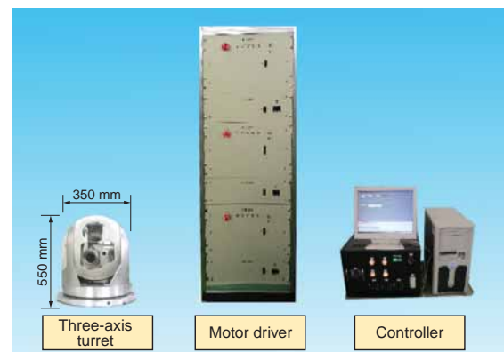
Three-axis turret for target tracking system
