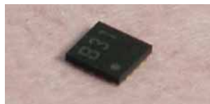
Low-noise amplifier IC (TQON16) External dimensions: 2.4 mm×2.4 mm×0.5 mm
