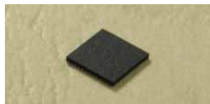
Receiver and transmitter IC (VQON44) External dimensions: 5.3 mm×5.3 mm×0.6 mm
