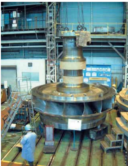
ランナと水車軸の組立て状態 Shop assembly of runner with turbine shaft
