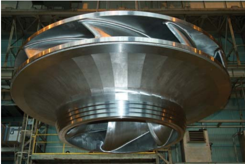
Splitter runner for Kannagawa Pumped Storage Power Station
