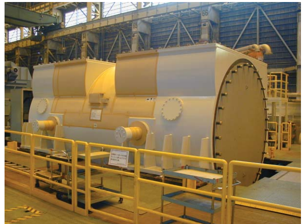
Generator stator ready for shipment
