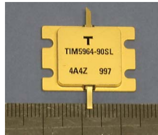
Micrographs of the package Package size: 24.5 mm×17.4 mm
