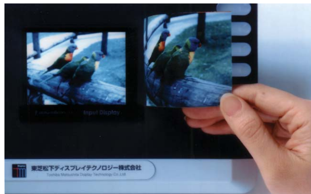
The world's first "input display" with color image capture function
