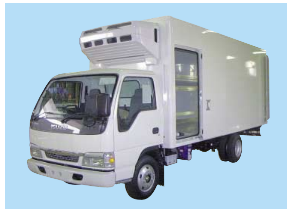
新型発電システム冷凍装置搭載冷凍車 Example of generator-driven refrigeration system installed on truck
