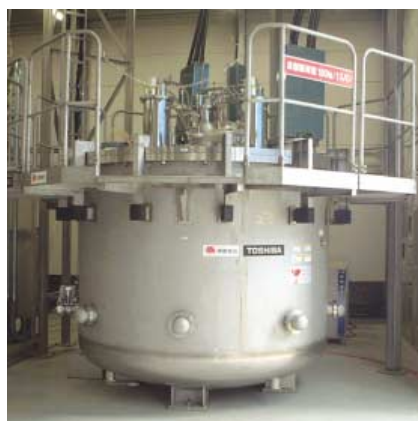
5MVA瞬低補償SMES用超電導マグネット Superconducting magnet of 5 MVA superconducting magnetic energy storage (SMES) system
