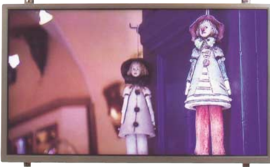
液晶TV用 22型WXGA OCBモード TFT-LCD 22-inch diagonal WXGA optically compensated bend (OCB) mode TFT-LCD for TV application
