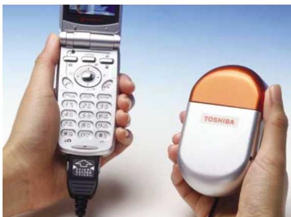
1W出力燃料電池(試作品) Prototype of 1W output direct methanol fuel cell (DMFC)
