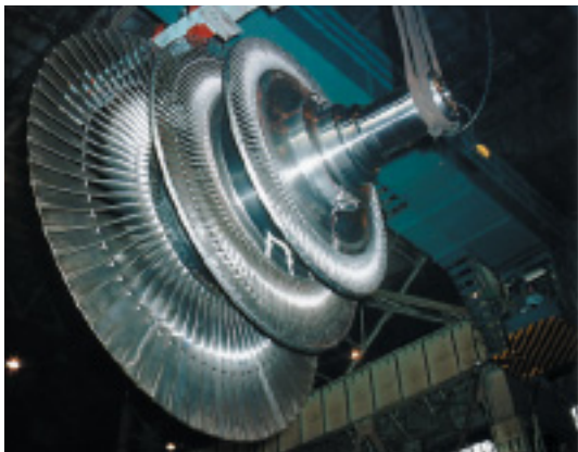
Series buckets of a steel 48-inch last-stage bucket (buckets and rotor for actual-size rotating test)
