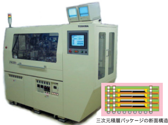
三次元積層パッケージ組立装置 3-dimensional stacked package assembly equipment
