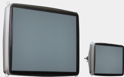
90 cm super large pure flat color picture tube (left) and 51 cm pure flat color picture tube (right)
