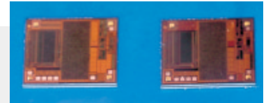
T6N81 LSI bare chip for RF-ID cards and tags
