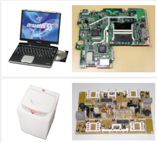
Notebook PC (top) and washing machine (bottom) manufactured with lead-free solder
